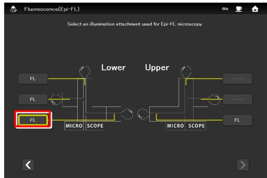
5. When the C-LEDFl is attached, select the wavelength of the light source used for epi-fl microscopy.
