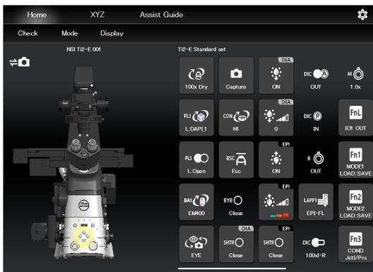
2. To switch the optical path, tap the target output port.
