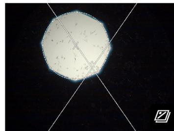
▼ **Optical axis adjustment (Example: Köhler illumination adjusted)**
