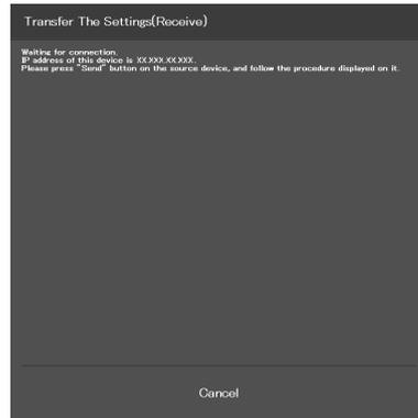
6. In the transmission terminal, enter the receiver's IP address displayed in step 5 in the [Destination IP address] field.
