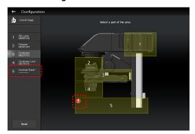
If transmission of the microscope configuration information is attempted in this state, a confirmation message for registering the part without device information to be [Unmount] appears.
