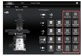
If the registered function buttons are not displayed in the remote control button area on the Home screen, change the display by selecting the relevant remote control button layout. For details, see "9.2.1 Remote Control Button Rearrangement."
