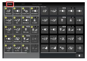
To save the customized button arrangement as a remote control button layout, specify a name in the [Name] field, and then tap [Save].
