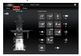
Select the [Microscope] tab and tap [Edit] of the desired mode number to save the mode in the microscope.
