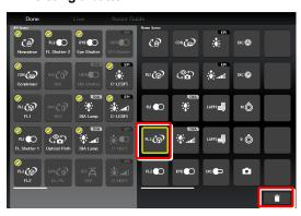
To delete multiple buttons at a time, first long-tap a button. After the yellow check mark appears on the top left of the long-tapped button, select the next button.
