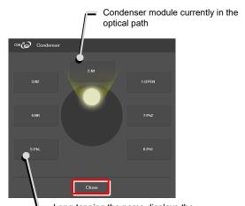
Long-tapping the name displays the detailed information about the condenser module.
