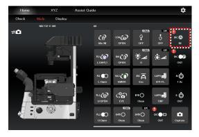
When all devices are in the states suitable for the registered mode, all the marks disappear and Mode in the menu field is shown in green.
