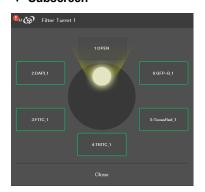
When all devices are in the states suitable for the microscopy technique, all the marks disappear and the microscopy technique in the menu field is shown in green.
