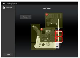
In a two-tier configuration, the upper and lower epi-illumination attachments are mounted in opposite directions. However, the application shows the two epi-illumination attachments in the same orientation.
