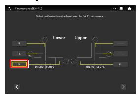
5. When the C-LEDFI is attached, select the wavelength of the light source used for epi-fl microscopy.
