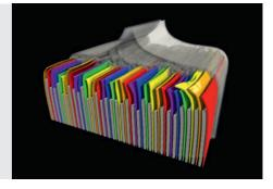
Lithium-Ion Battery Pouch Cell [scanned with Half.Turn CT] ▶
