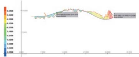
Able to obtain sample cross-sectional shapes with the high-speed laser scan at 1000 points per second. Compatible with shape evaluation in height direction.
