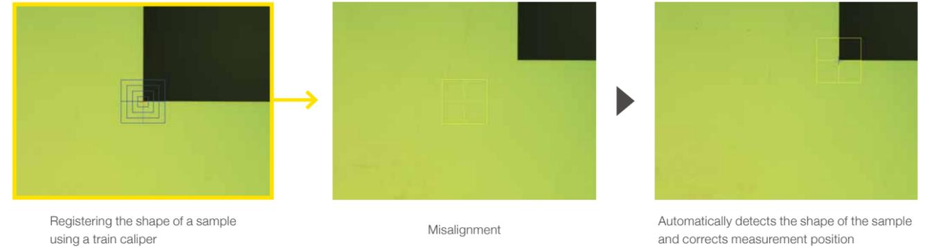
Using 3D images, it is also possible to automatically detect and measure bumps and bonding wires that are misaligned from their designed positions.
