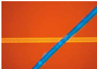
Epi-fluorescence observation of organic substance on wafer
