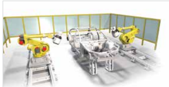
Metrology room: Using APDIS in the metrology room as a replacement for traditional CMMs, the off-line facility ceases to be a bottleneck due to faster measurements allowing quicker problem investigation.
