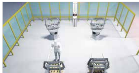
Component inspection: Incoming part inspection is critical to avoid assembly issues further down the production line. The APDIS Laser Radar allows for fast, non-contact feature and surface inspection on components from doors to bodysides, to have an instant quality report on components from external suppliers.
