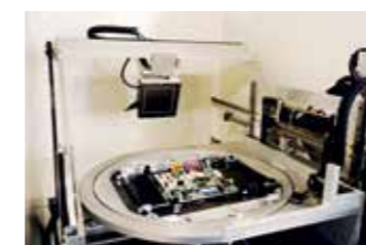
Under any combination of rotation, tilt and magnification, the region of interest is consistently locked into the center of the field of view
