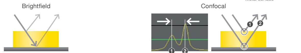
Unstable reflection makes it difficult to detect the exact location
