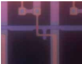
No correction for cover glass thickness (with 50x objective lens)
