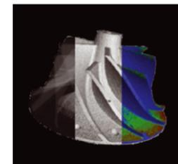
3D printed impeller
