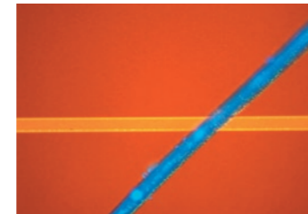
Epi-fluorescence observation of organic substance on wafer
