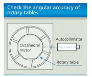
Measure the accuracy of rotary tables or dividing heads using polygon mirrors.
