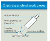
Measure the difference between the crosshair images reflected from the end surface of the work piece and from a standard angle block.
