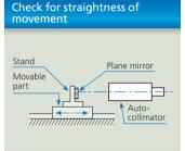
Attach a plane mirror, either directly or on a stand. to the moving part and read deviation from the reflection.
