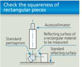
Compare the reading difference between the standard reflecting surface and the surface of the specimen using the Pentaprism.
