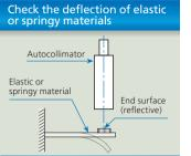
Affix the mirror the specimen and read the angular deflection using the autocollimator. Small vibrations may also be detected in this manner.
