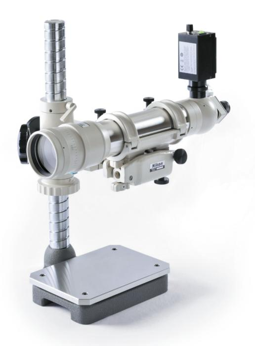
An easy-to-use, precise metrology instrument for angularity, parallelism, perpendicularity, straightness of precision components, machine guide-way and many other applications.
