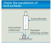
Compare the difference between the crosshair images reflected from the surface of the specimen and from a standard surface.
