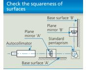
Compare the readings taken from plane mirror 'a' on surface 'A' to those from plane mirror 'b' on surface 'B' through the Pentaprism.
