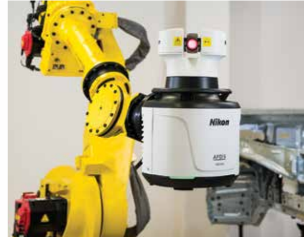
APDIS Laser Radar mounted on a robot is an innovative alternative for a traditional horizontal arm CMM
