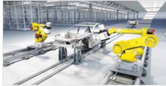
Inline inspection: the APDIS MV430E provides the fastest feature measurements of any Laser Radar, allowing inspection of critical features directly within the production line
