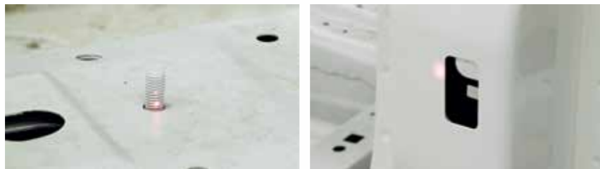
Features like holes, slots, pins, studs etc are inspected in an automated way with precision scan paths and optimized data sets.
