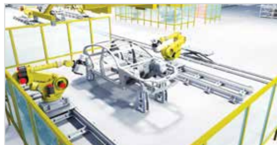
Bypass inspection: By automatically removing a car body from the line, detailed inspection is possible on vastly more components than previously possible. After inspection, the body is automatically re-inserted into the production line for seamless integration.
