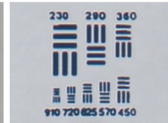
Resolution chart (Objective: TU Plan Fluor 10x)
