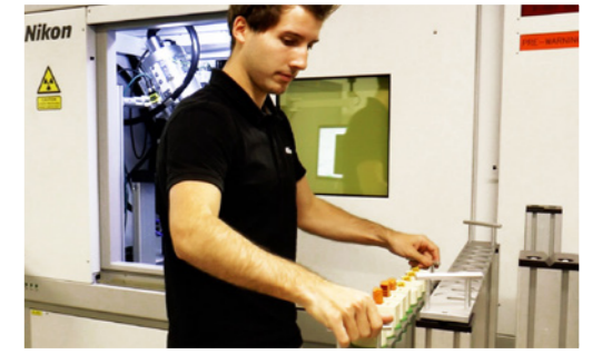
Loading the sample part holder in the CT system
