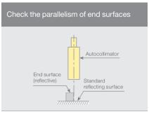
Compare the difference between the crosshair images reflected from the surface of the specimen and from a standard surface.
