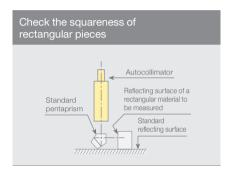
Compare the reading difference between the standard reflecting surface and the surface of the specimen using the Pentaprism.
