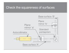
Compare the readings taken from plane mirror 'a' on surface 'A' to those from plane mirror 'b' on surface 'B' through the Pentaprism.
