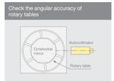
Measure the accuracy of rotary tables or dividing heads using polygon mirrors. The octahedral mirror measures in units of 45°, and the dodecahedral mirror in units of 30°.
