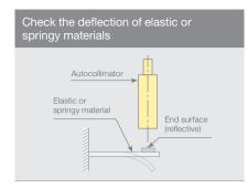
Affix the mirror the specimen and read the angular deflection using the autocollimator. Small vibrations may also be detected in this manner.
