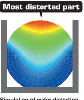
Simulation of wafer distortion
