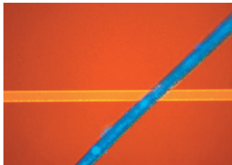
Epi-fluorescence observation of organic substance on wafer
