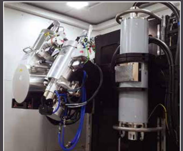
Triple source combination with 225 kV rotating target, 450 kV high-brilliance and minifocus source.
